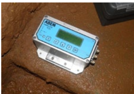
Obr. 5. Vibrograf ABEM Vibraloc použitý na meranie technickej seizmicity (Pandula a Kondela, 2021) Fig. 5. Vibrograph ABEM Vibraloc used for measuring of technical seismicity (Pandula and Kondela, 2021)
