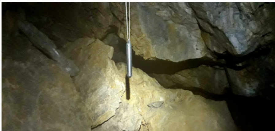
Obr. 2. Logger na meranie teploty a tlaku vzduchu. Stanovište 3. Foto: L. Pristašová Fig. 2. Logger for the measurement of air temperature and pressure. Station 3. Photo: L. Pristašová
