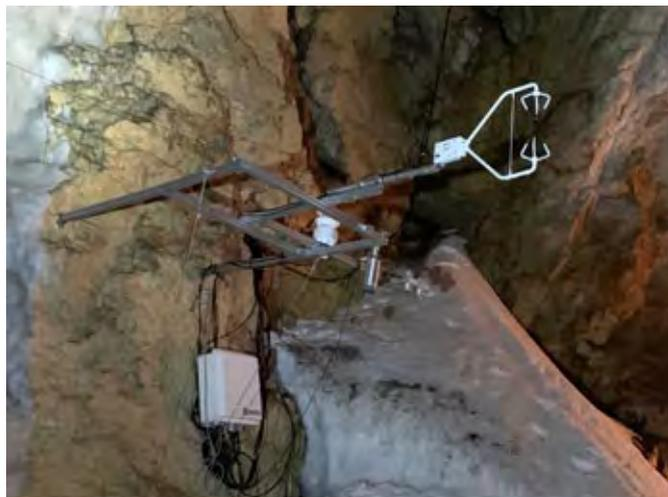
Fig. 1. Meteorological monitoring station at Hundalm ice cave. Photo: C. Spötl
