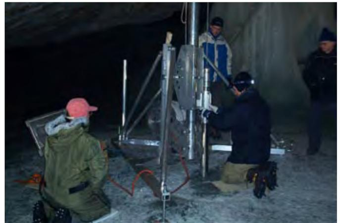
Fig. 7. Deep drilling into the ice of the Great Hall using a special drilling set made by experts from the University of Bern for the isotope study, geochemical study, and dating of ice. Photo: J. Zelinka
