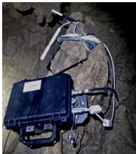
Obr. 2. Mobilná stanica na meranie a monitorovanie jaskynnej klímy. Foto: L. Kunáková Fig. 2. Mobile station for measurement and monitoring of cave climate. Photo: L. Kunáková
