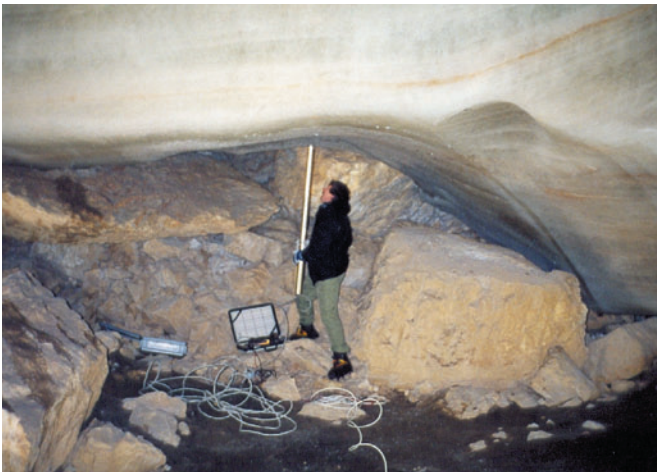
Fig. 5. Sampling with the hand held drill at the bottom of the Cave
