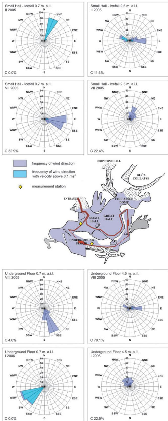
Fig. 4. The Frequency of the direction of air flow measured at points between Small Hall and Icefall (0.7 m a.i.l. and 2.5 m a.i.l.) and in Underground Floor (0.7 m a.i.l. and 4.5 m a.i.l.) in chosen summer and winter months
