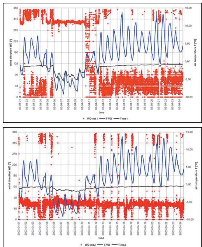
Fig. 7. The temporary changes of air exchange course measured in April 2003 at measurement points localised in Small Hall area on the height of 0.7 m a.i.l. (a) and 3.0 m a.i.l. (b) against air temperature changes inside ( $T_{\text{ms1}}$ ,  $T_{\text{ms2}}$ ) and outside ( $T_{\text{VO}}$ ) the cave
