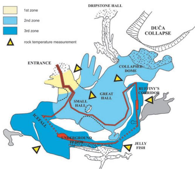
Fig. 9. The division of the cave on zones in terms of potential conditions of ice crystals sediments formation
